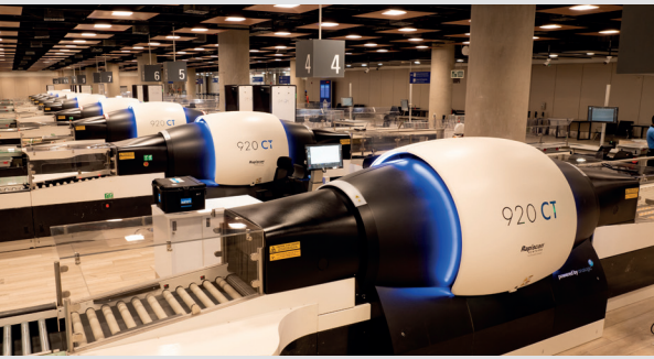
27 inspection lines with CT scanners offering 360° imaging—no need to remove liquids or electronic devices.
